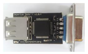
Orientation of the Imperium Solo when setting the jumpers. USB port left and Joyport right.
